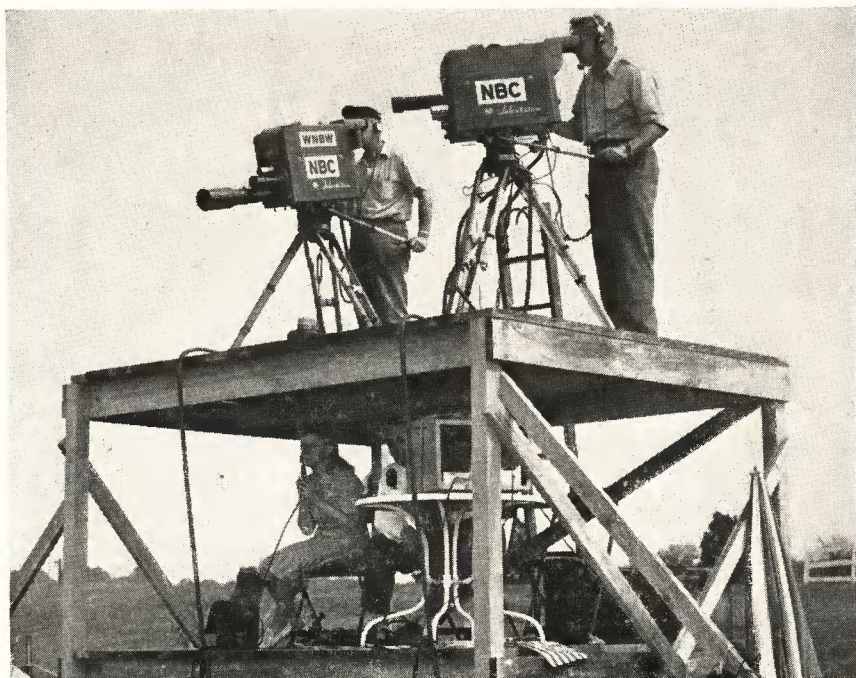
WNBW-NBC, Wash. D. C., erects platform for cameras to cover outdoor events, especially horse shows. Note director and ass't beneath platform for view of action and monitors.
